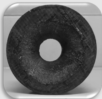
Rocket nozzle after test showing near zero erosion in the throat and chamber pressure during the test
