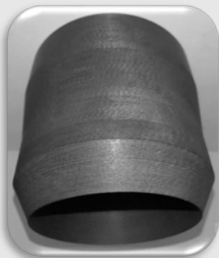
100 mm long rocket nozzle machined from a UHTCMC blank
