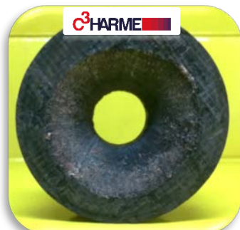
Rocket nozzle after test showing near zero erosion in the throat
